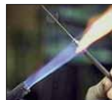
Retipping a Firing Pin
